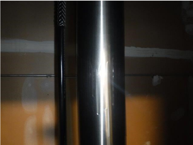
1. Check piston and packing.
